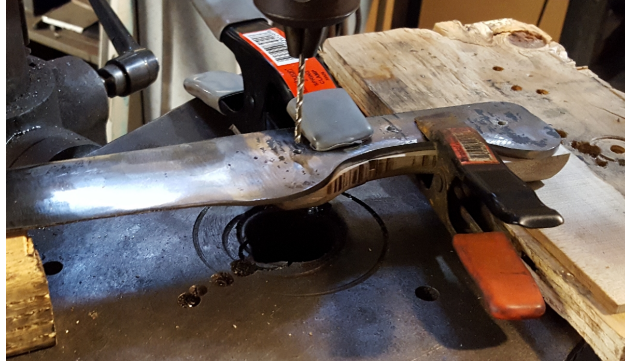
Figure 5.33.: Drilling the wood using the other holes as guides.
