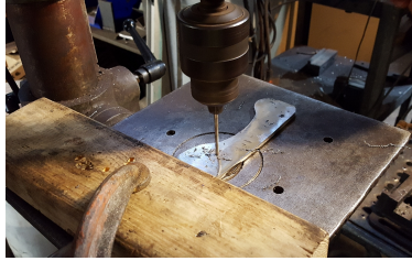
Figure A.16.: Drilling through the tang for the pins.
