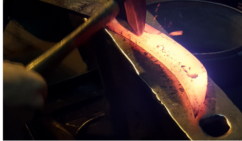
Figure 5.17.: Using the cross-peen hammer to stretch out the width of the blade.
