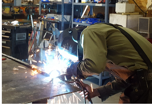
Figure 5.8.: Josh tack welding the bars together.
