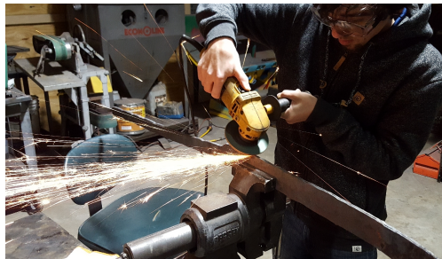
Figure A.7.: Grinding the edges to see the weld quality.
