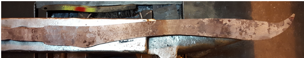
Figure 5.19.: The shape of the sword after most of the forging on the blade.
