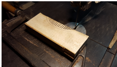
Figure A.14.: The perpendicular pre-cuts.
