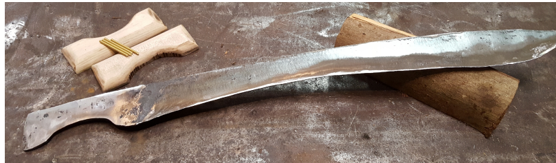
Figure 5.27.: The blade with most of the scale cleaned off. The wooden pieces and the pins of the handle are on the upper left.
