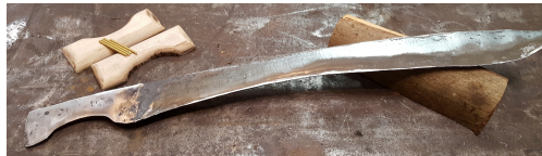
Figure A.11.: The blade with most of the scale cleaned off. The rough pieces of the handles and the pins are on the upper left.
