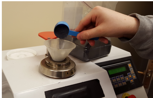
Figure 6.13.: Amount of material needed for mounting the metal sample, as well as proper delivery techniques.
