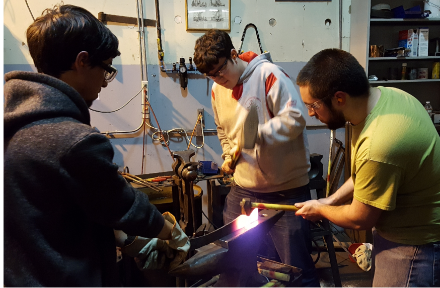
Figure 5.21.: The 3-person layout used to shape the tang more rapidly.
