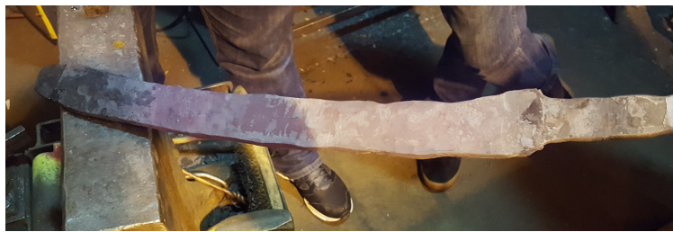
Figure 5.13.: The result after lamination.
