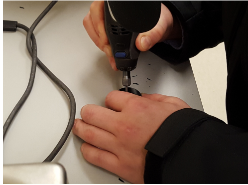
Figure 6.15.: Process used to mark/scribe the samples post-mounting.
