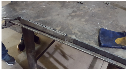
Figure 5.9.: The results from the tack weld.
