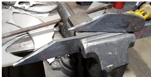
Figure 5.15.: The cut on the end to make an angle and get a piece for the sample.
