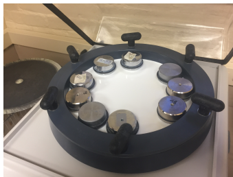
(a) The polishing tray with abrasive solution and samples.
