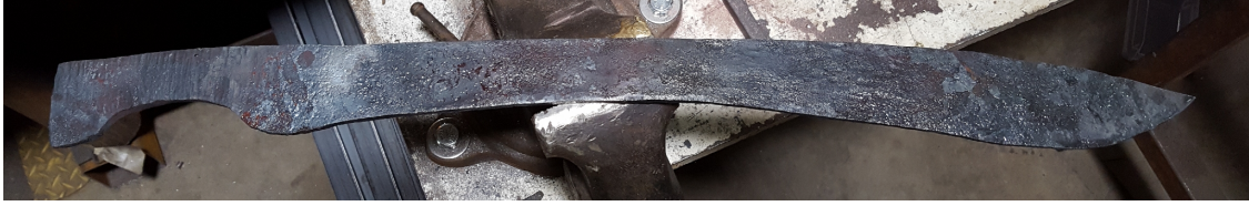
Figure 5.22.: The end of the forging process, with the fully shaped tang.
