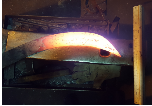
Figure 5.16.: The counteractive bend (with a scale).
