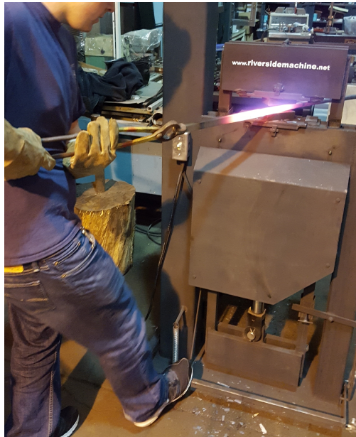
Figure 5.5.: The hydraulic press used for major flattening processes.
