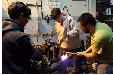
Figure A.12.: The 3-person layout used to shape the tang more rapidly.
