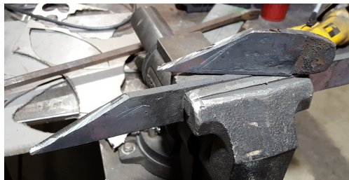
Figure A.8.: The cut on the end to make an angle and get a piece for the sample.
