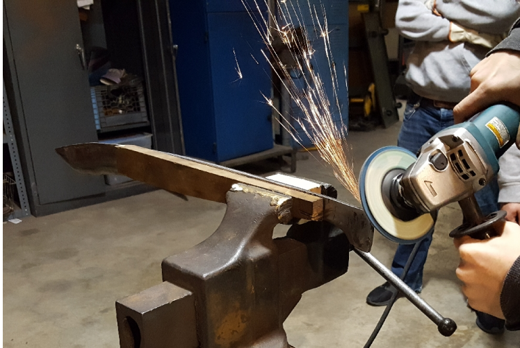
Figure 5.25.: Smoothing out the edges and thin parts of the blade.
