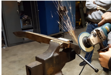
Figure A.13.: Smoothing out the edges and thin parts of the blade.
