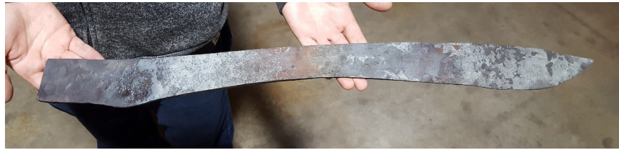
Figure 5.20.: The shape of the sword after cutting off extra material on both ends.
