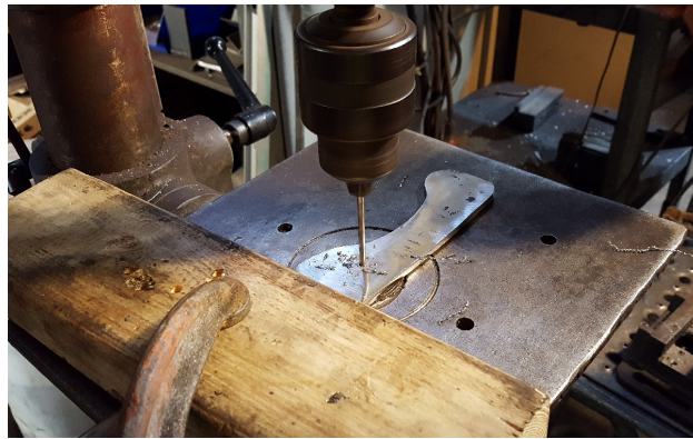
Figure 5.32.: Drilling through the tang for the pins.
