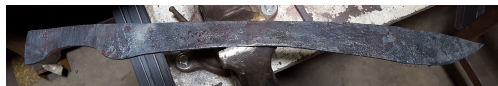
Figure A.10.: The end of the forging process, with the fully shaped tang.
