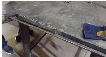
Figure A.4.: The results from the tack weld.
