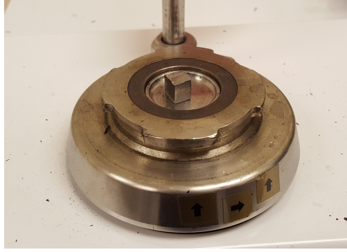
Figure 6.12.: The tray used to mount samples, as well as the proper positioning for a sample.
