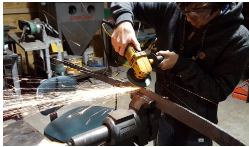
Figure 5.14.: Grinding the edges to see the weld quality.
