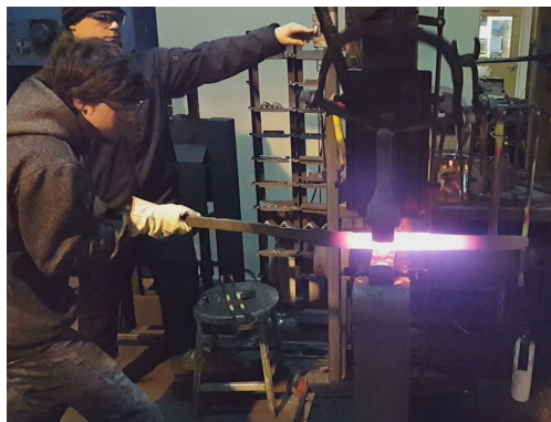
Figure 5.12.: The power hammer used to efficiently laminate the metals.
