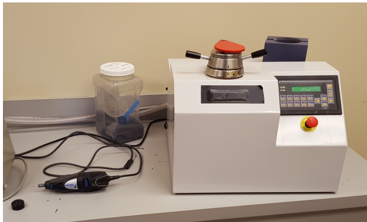
Figure 6.11.: The machine used to mount the steel samples.
