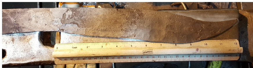
Figure 5.18.: The end of the sword after the majority of the stretching was completed.
