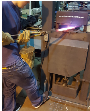
Figure A.3.: The hydraulic press used for major flattening processes.
