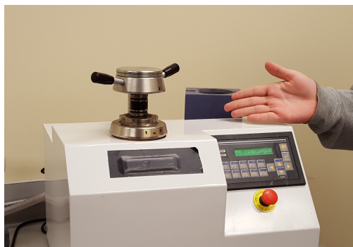
Figure 6.14.: The sample as it leaves the mounting press.
