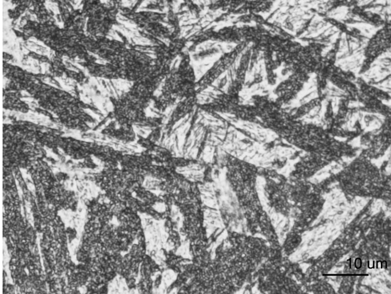
Figure 44: Microstructure of forged 4140 steel blade.
