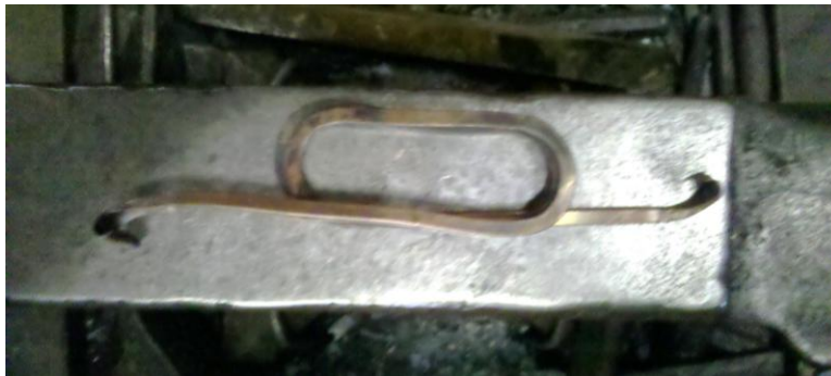
Figure 33: The finished crossguard.
