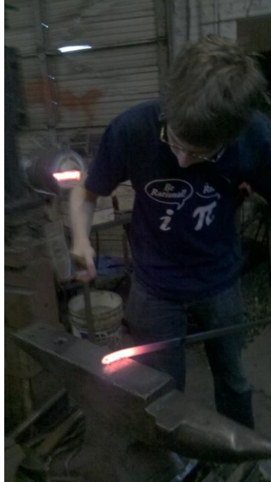
Figure 24: Forging the tip of the blade.
