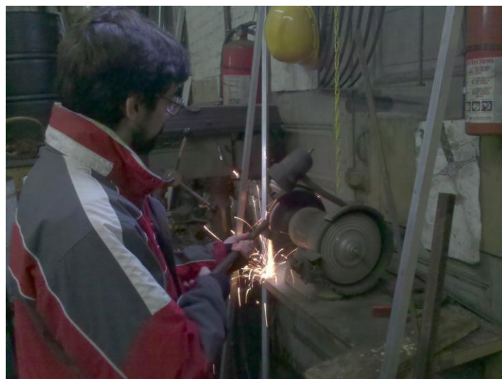
Figure 40: Preparing the pommel for forging.
