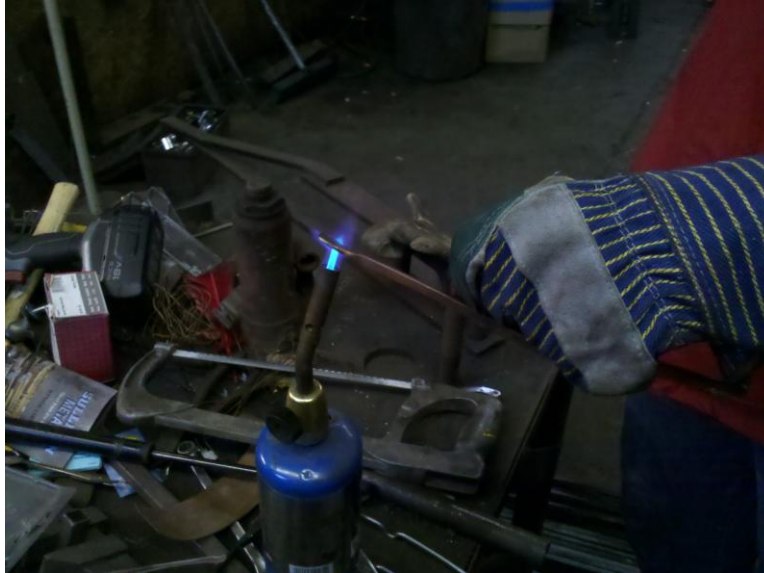
Figure 32: Annealing of the crossguard.
