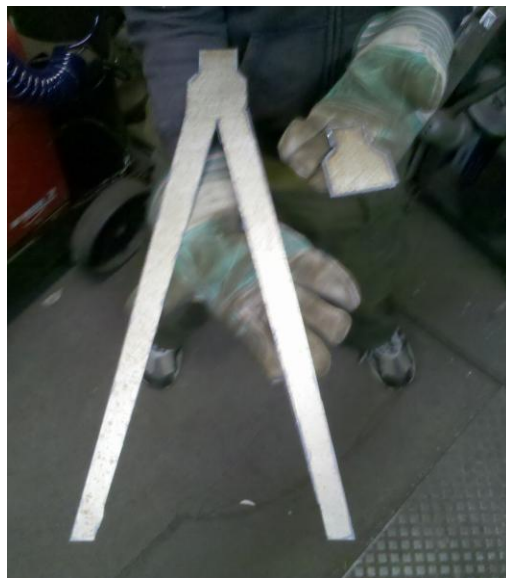
Figure 38: Finalized knuckle guard cutouts.
