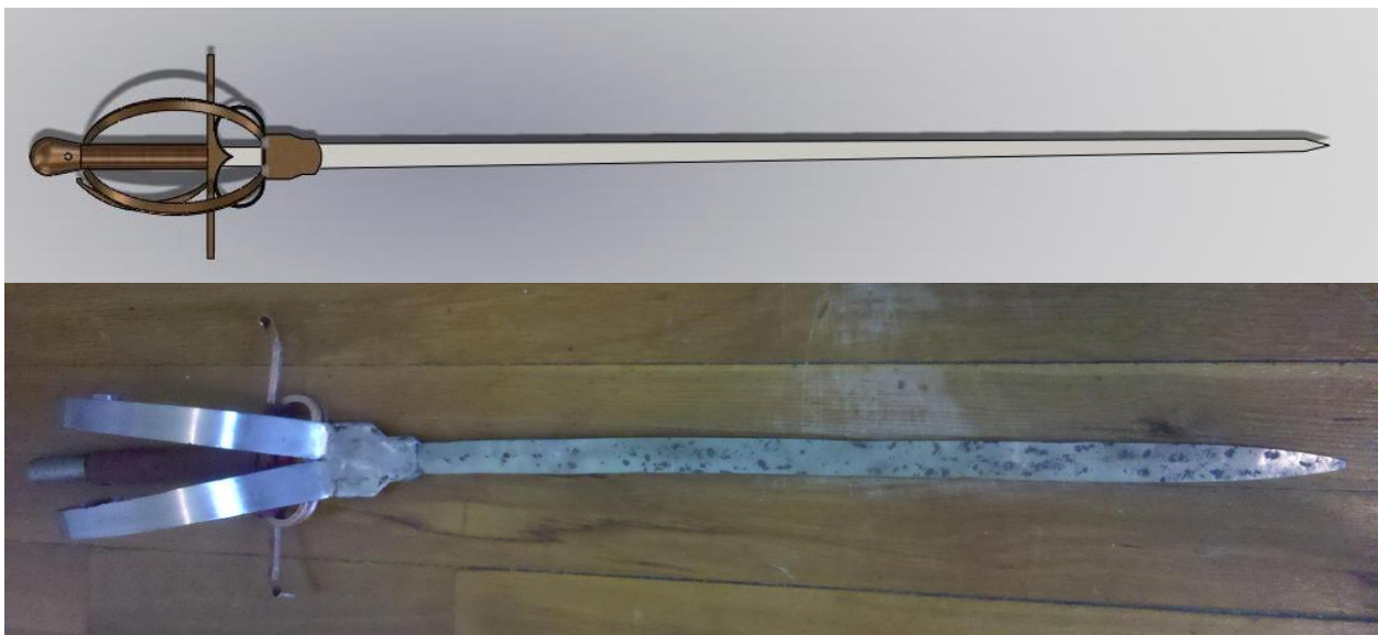
Figure 38: Comparison of the CAD model rapier (top) and the hand manufactured rapier (bottom).
