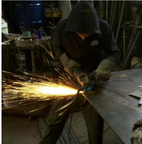
Figure 37: Removing rough edges from the guard pieces.
