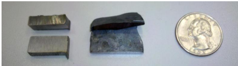
Figure 20: The steel samples with quarter for scale. Left: Unforged steel. Middle: Heated and shaped steel.
