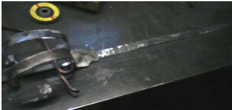
Figure 39: The finished knuckle guard.
