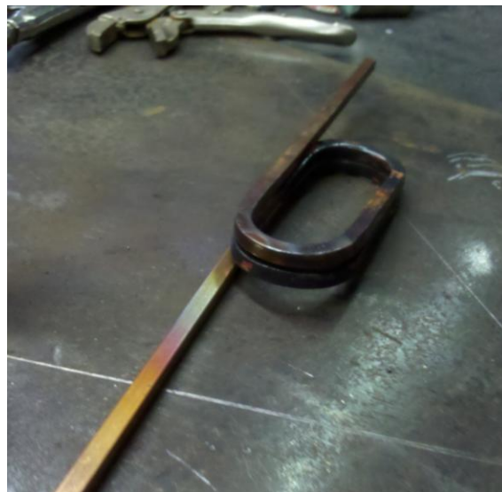
Figure 31: The crossguard after being coiled.
