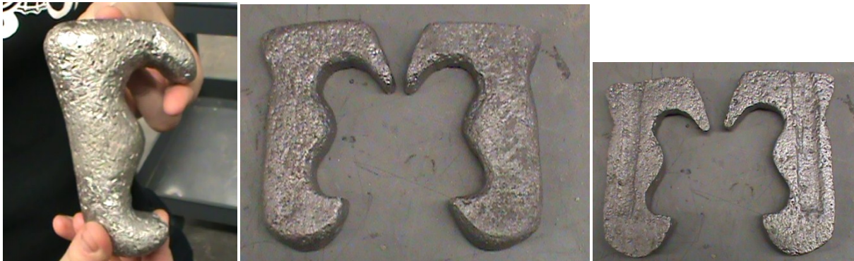
Figure 58: (Left) Finished Practice Run Handle, (Right) Finished 2 Halves of Final Actual Handle.
