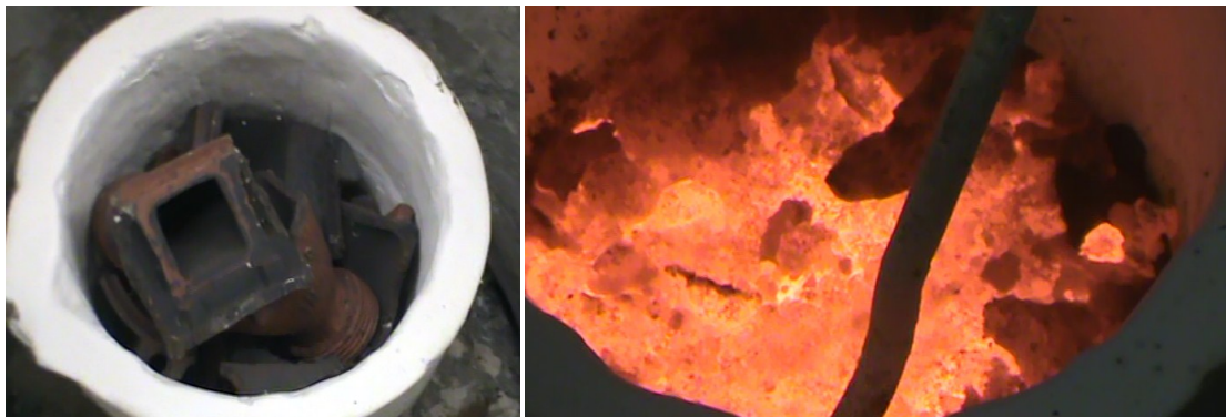
Figure 52: Bronze Pieces Placed Inside Crucible within Furnace (Before and After).
