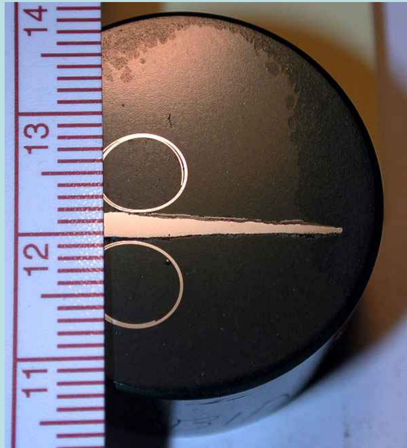
Column Section Showing Region with Severe Thinning
