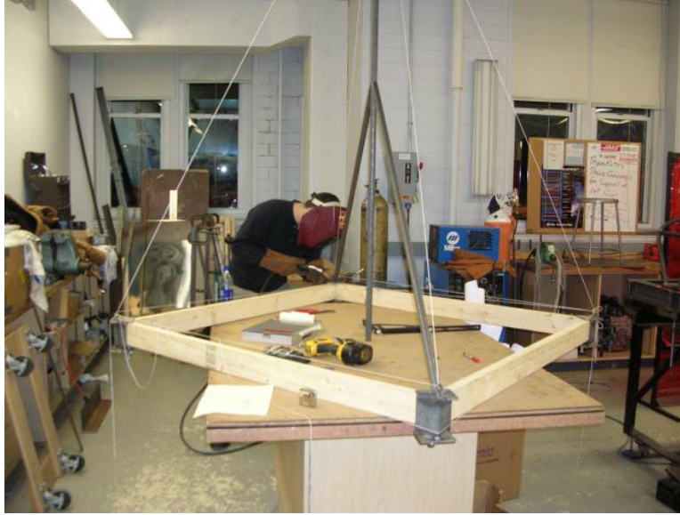
Figure 25: Wooden Jig Constructed, Corner Bracket Being Welded
