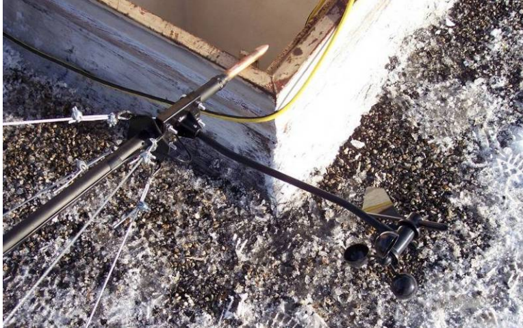
Figure 29: Copper Electrode and Weather Station Affixed
