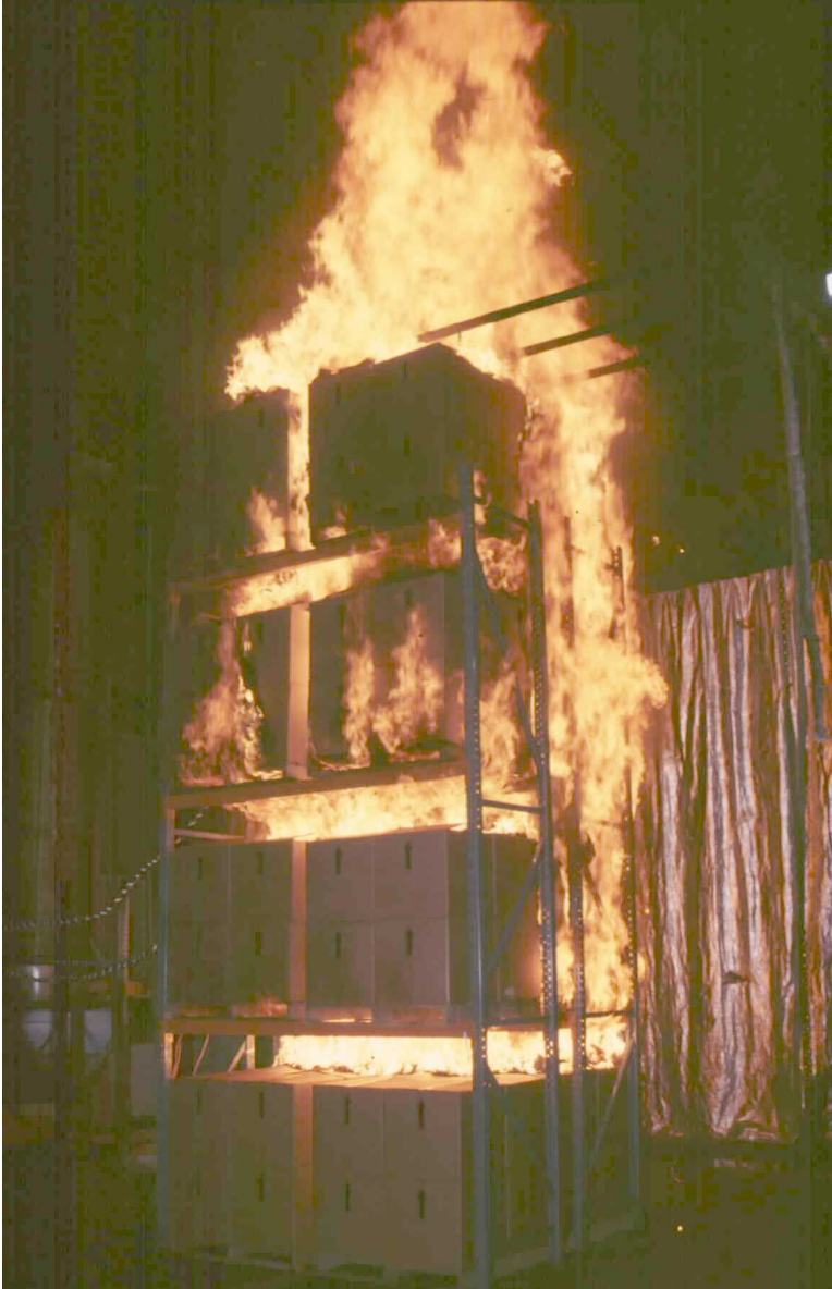
FIGURE 2: Photograph of a rack storage fire, courtesy Underwriters Laboratories, Northbrook, IL.
