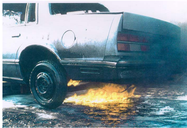
Figure 3. Dripping and pooling underbody gasoline fire suppressed by SPGG.
