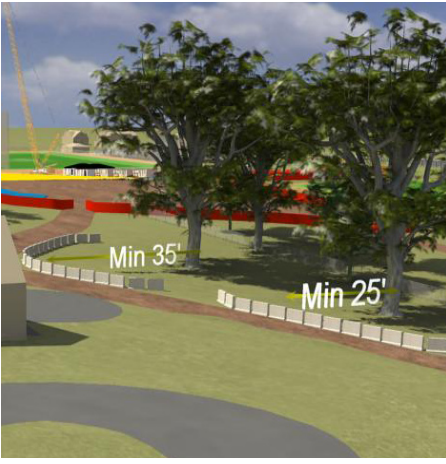
Gilbane’s BIM model showing the 25-foot clearance required to protect WPI’s valuable trees near the site.
