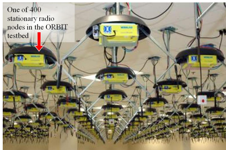
Figure 7: The indoor testing facility at Rutgers University [21] is open for use to members of the research community who write their own code. Each yellow box is one of 400 stationary radio nodes.
