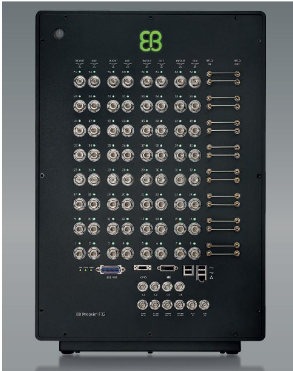
Figure 11: Elektrobit Prosim F32, radio channel emulator [24]. The F32 model has the capacity to support as many as 32 distinct RF channels with 16 bidirectional nodes. This channel emulator can also simulate fading.
