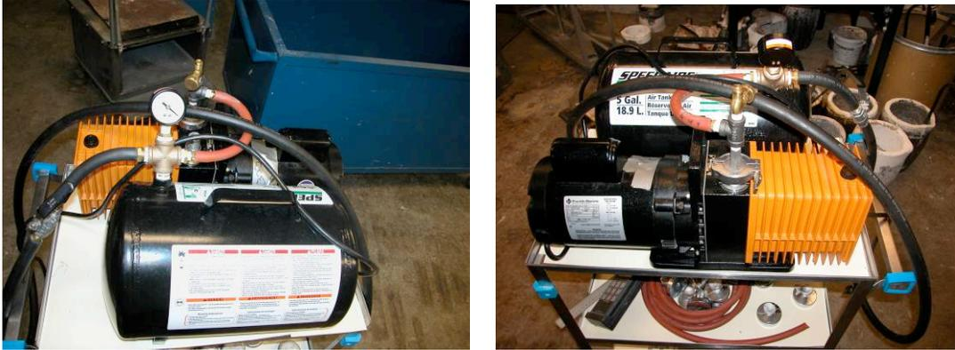
**Figure 3.2.1.A, B:** Pressure testing setup, including air tank, 1/2 hp pump, gauge, valves. Front (A) and Rear (B).
