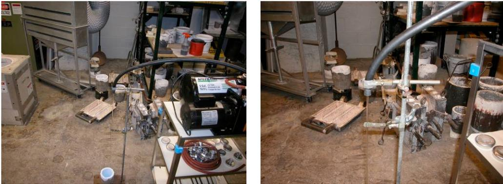
**Figure 3.2.1.C,D:** C) Lab stand, borosilicate tube, and crucible in upright position. D) Close-up of borosilicate tube, stand, rubber tube, and rubber stopper in lower position.
