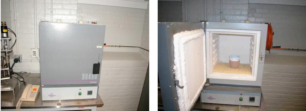
**Figure 3.2.1.G,H:** Resistance heated furnace (G), used to preheat crucibles (H)
