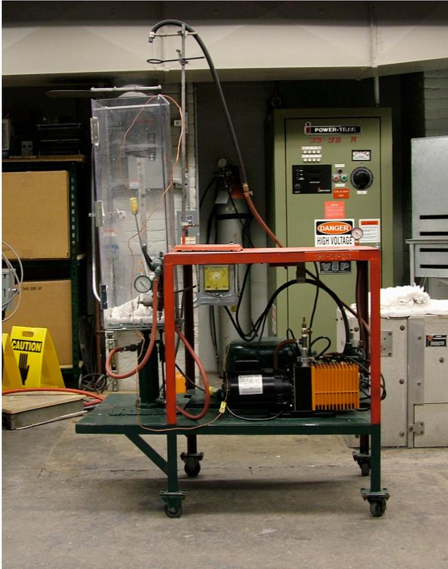
**Fig. 3.2.2.A: Vertical vacuum apparatus in the lab foundry**
