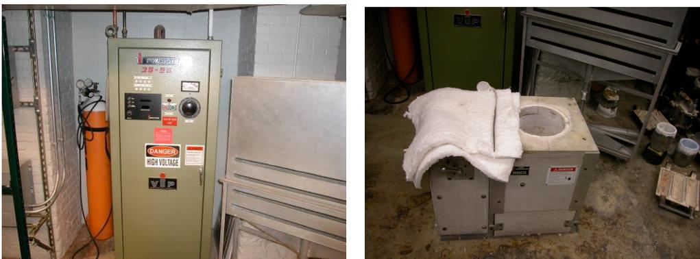
**Figure 3.2.1.E,F:** E) Induction unit controls and F) induction unit
