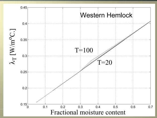
Transverse diffusion coefficient for the heat diffusion process as a function of moisture and temperature. Temperatures in degree C.
