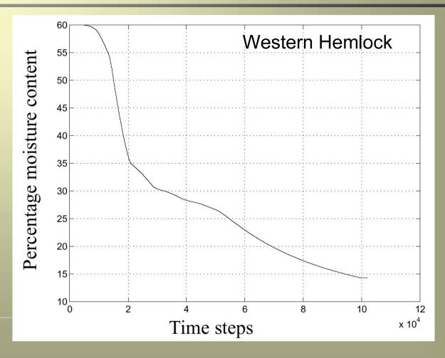
Evolution of moisture content in the center of a wood sample when RF energy is applied
