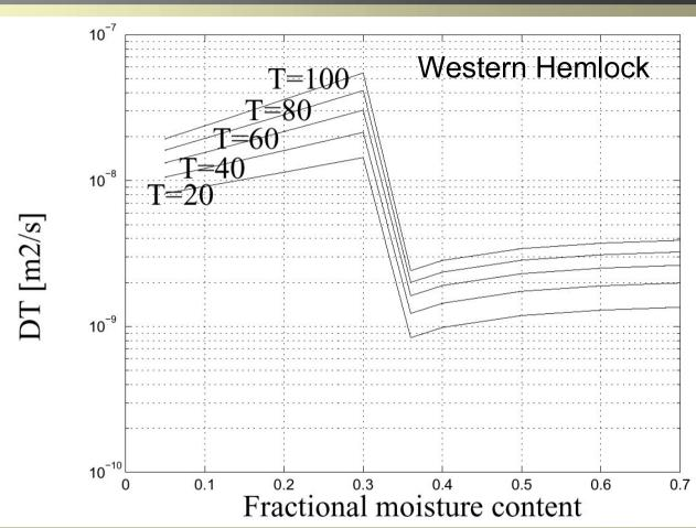
Transverse diffusion coefficient for the moisture diffusion process as a function of moisture and temperature. Temperatures in degree C.
