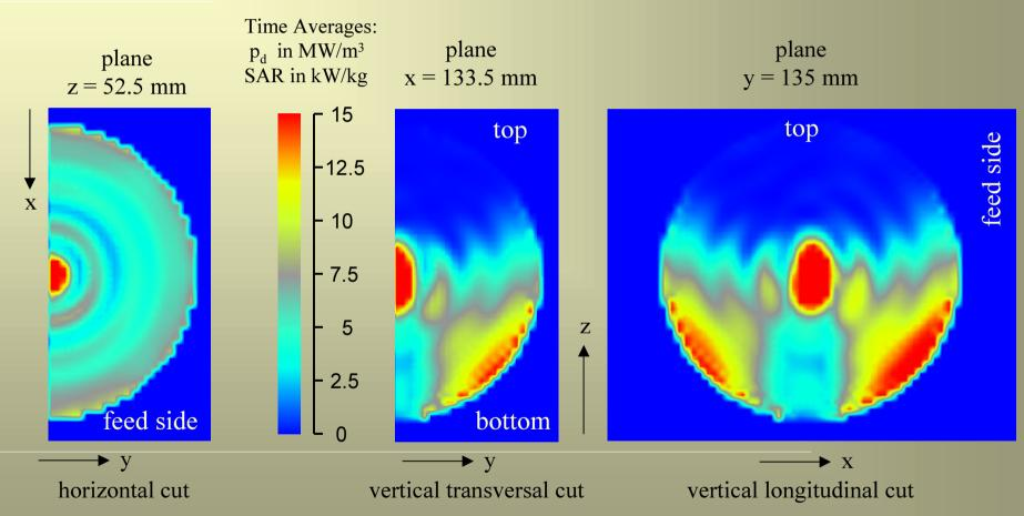
Density of average dissipated power  $(p_d)$  and SAR in the potato 1 kW magnetron matched to the waveguide, f = 2.45 GHz, steady state
