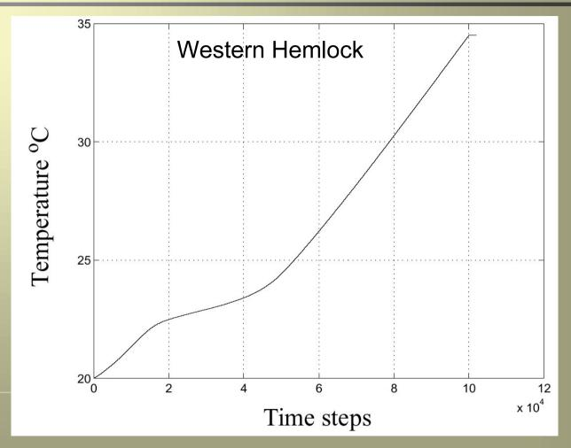
Evolution of temperature in the center of a wood sample when RF energy is applied
