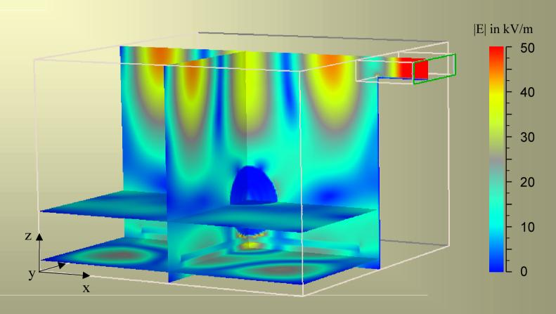
Envelope of the peak value of the electric field  $|E|_{max}$  1 kW magnetron matched to the waveguide, f = 2.45 GHz, steady state
