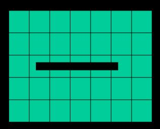
Thin slots can be modeled at a sub-cell level Slots can be open or filled with a material to represent gaskets Overlapping or butted joints Slot bends and junctions
