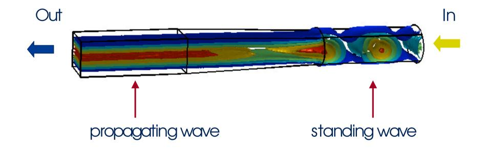
• The incoming TE11-mode is transformed to a TE10-wave
