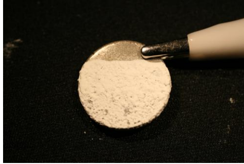
Fig. 1. Metallic powder compact (grey region) electrophoretically coated by a “green” zirconia particle (white region) coating.
