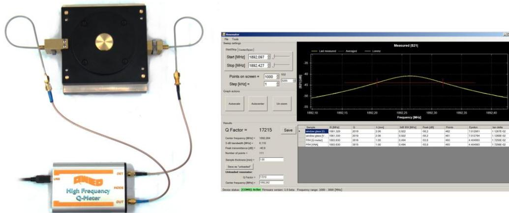
Fig. 2. System running with 1.8 GHz resonator.
